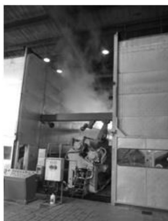
Slika 2. Gubici toplote sa papir mašine u prostor proizvodne hale kod lajm prese Figure 2. Heat losses from the paper machine to the production hall space at the lime press.
