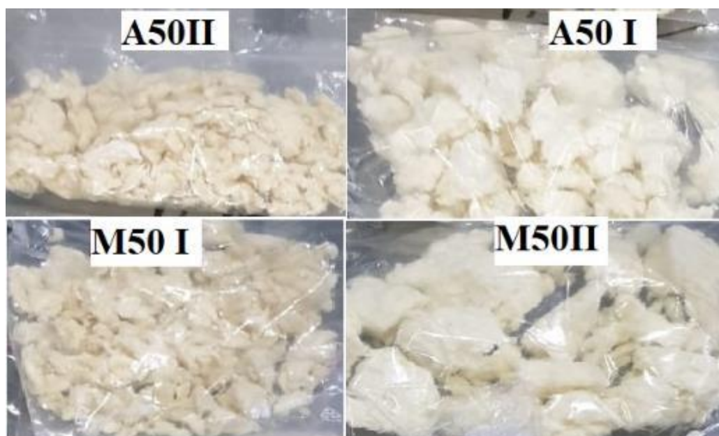
Fig. 3 Eucalyptus thermomechanical pulp bleached with POM catalyst
