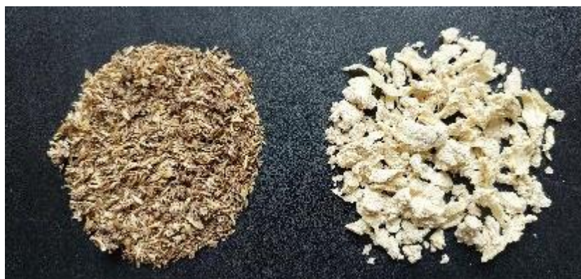
Fig. 6 Cellulose from brewing malt bleached with polyoxometalate catalysts.
