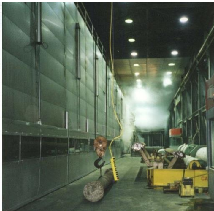
Slika 1. Formiranje magle u zoni mokrog dela papir mašine [3] Figure 1. Formation of mist in the wet-end zone of the paper machine [3].
