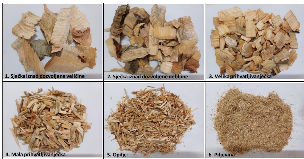
Slika 3: Prikaz frakcija sječke prema SCAN 40:01 Figure 3: Distribution of wood chip fractions according to SCAN 40:01
