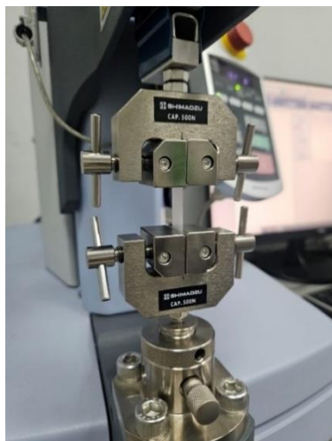
Figure 2: A sample, strip of double-layer BNC/PVDF film was placed in the jaws of the tensile testing machine Slika 2: Uzorak, traka dvoslojnog BNC/PVDF filma, postavljena je u čeljusti kidačice
